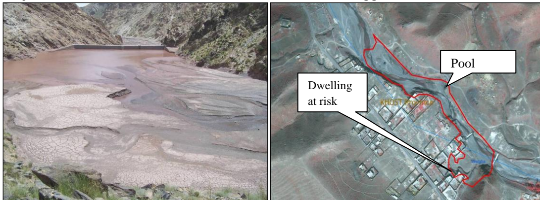
Figure 7. Reservoir Filling on a Large, Unstable Stream (Oosterkamp) and Inundation.
