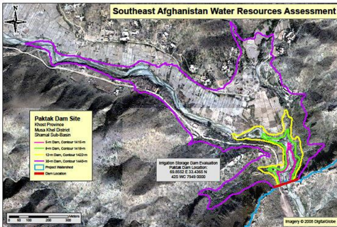
Figure 10. Reservoir Inundation Map, Paktak Dam, Khost
