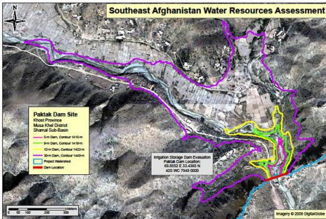
Figure 10. Reservoir Inundation Map, Paktak Dam, Khost
